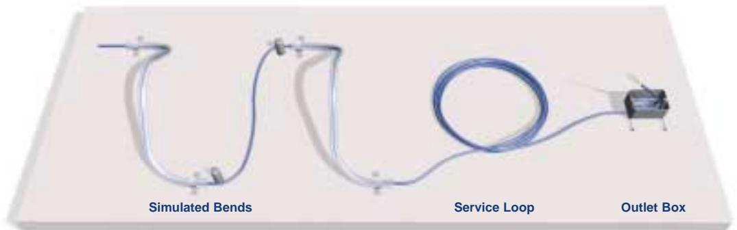
**Installation Stress Test Set-Up**
